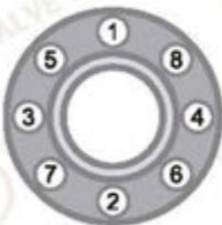
When installing flanges, it is critical that bolts be equally tightened in sequence which diametrically opposed to each other.
